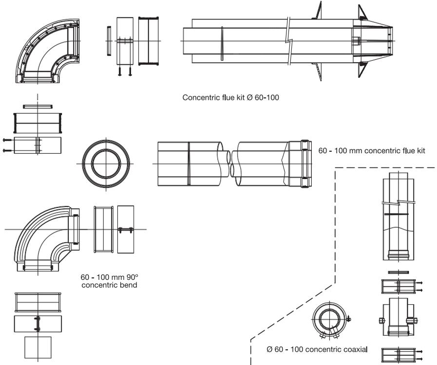
If the length of the pipe is 1 metre or less, the diaphragm (inner  $\varnothing$  85 mm) supplied in the accessories bag should be fitted.
