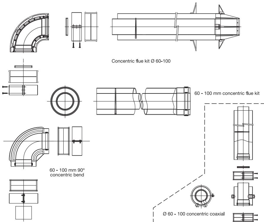
If the length of the pipe is 1 metre or less, the diaphragm (inner Ø 85 mm) supplied in the accessories bag should be fitted.
