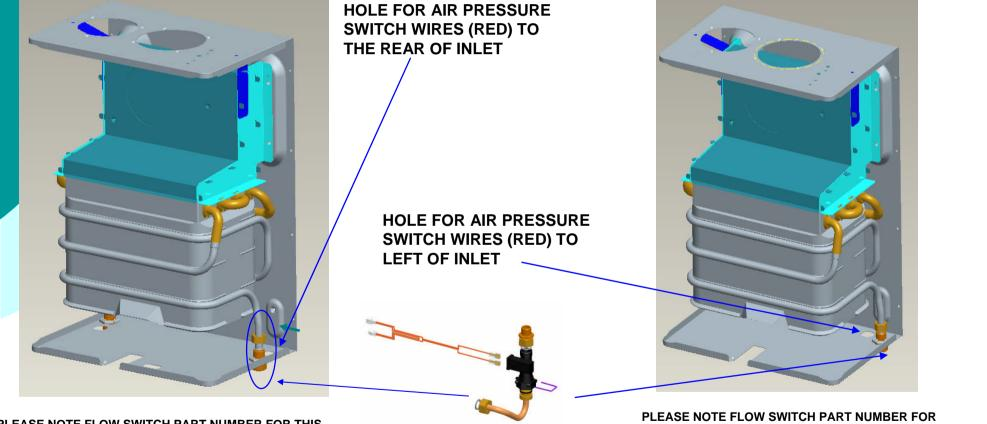
PLEASE NOTE FLOW SWITCH PART NUMBER FOR THIS HEAT EXCHANGER IS (MRS0220) SUITABLE FOR HEATERS WITH SERIAL NUMBERS ENDING 0000 -0937
