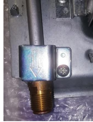
2. Fit the Heat Exchanger bracket above the brass racord as shown
