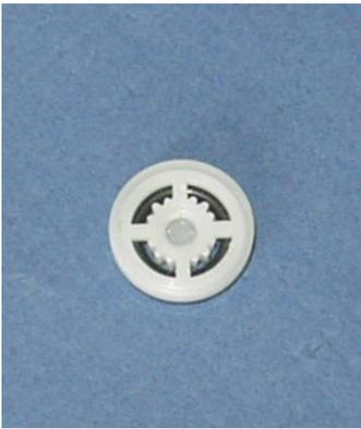
MCB2240 - Flow Regulator – this is fitted inside the combi on the cold water inlet. It cannot usually be seen unless the cold water inlet system is removed from the inside of the combi. This is usually a job for an experienced engineer. It is about the diameter of a penny and is easy to lose or forget when re-assembling a boiler and this may explain why they can be missing.
