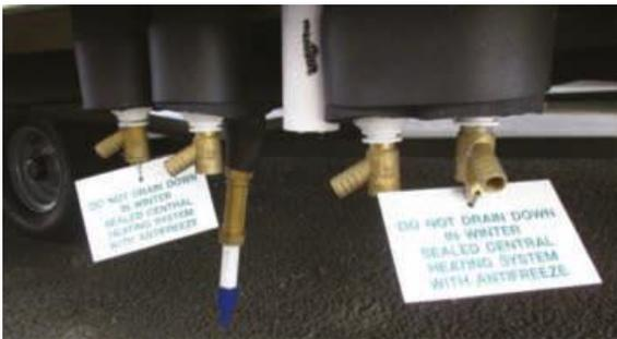
This manufacturer has helpfully labelled the central heating system drain cocks to avoid them being incorrectly used.
